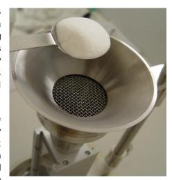
Re-weigh the cup and calculate the weight of the collected powder sample. Now use the known volume of the cup to calculate the apparent density. This can be done using the formula:
