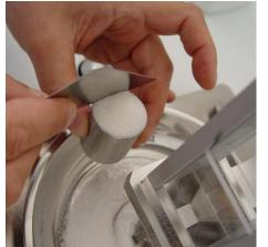
until the cup beneath overflows. Now level off the powder using a flat edge scraper.
