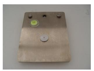
The design is made from a solid stand and a horizontal, vibration free baseplate including an integrated spirit gauge to check the levelness of the instrument, a stainless steel cylindrical cup, bottom and top funnel, a baffle box, spatula and brush.
