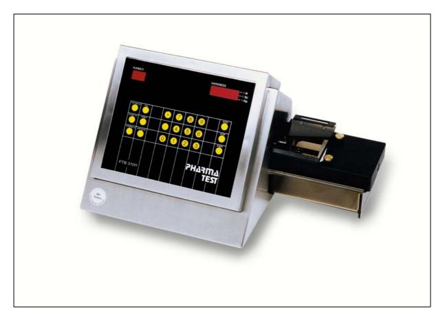
The Manual Tablet Testing Instrument **PTB 111E** is a **dual** force mode hardness test apparatus as it can be used for either linear force or linear speed increase while Tablet Hardness is tested. It offers a multiple point validation procedure for the built-in digital load cell.
