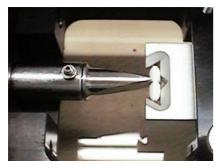
The specially designed sample holder and force jaw is suitable to be used in the PTB 111E Testing Instrument. It is designed to test the tension strength at the break line of shaped and also round tablets
